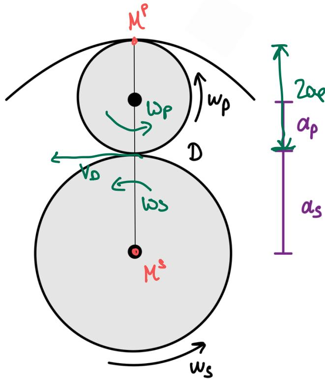
$$V_0 = \omega_s a_s \stackrel{!}{=} -\omega^2 a_p$$
