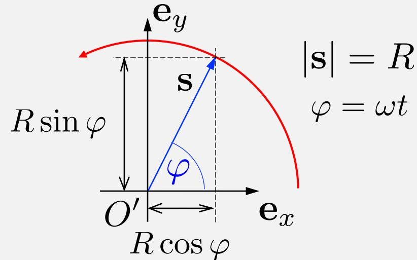
$$x(t)^2 + y(t)^2 = R^2 \cos^2 \omega t + R^2 \sin^2 \omega t = R^2 (\cos^2 \omega t + \sin^2 \omega t) = R^2$$
