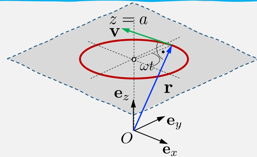
$$\begin{aligned}\mathbf{v}(t) \cdot \mathbf{r}(t) &= \mathbf{v}(t)^T \mathbf{r}(t) = \begin{bmatrix} -R\omega \sin \omega t & R\omega \cos \omega t & 0 \end{bmatrix} \begin{bmatrix} R \cos \omega t \\ R \sin \omega t \\ a \end{bmatrix} = \\ &= R^2 \omega (-\sin \omega t \cos \omega t + \sin \omega t \cos \omega t + 0) = 0\end{aligned}$$
